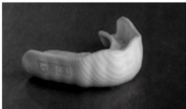
Fig. 2: GRiTT 3D creating custom 3D printed sports mouth guards.
